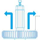
Unique, innovative heat sink and vertically mounted driver allows airflow through the entire unit, pulling heat away from the LED chips and driver.
